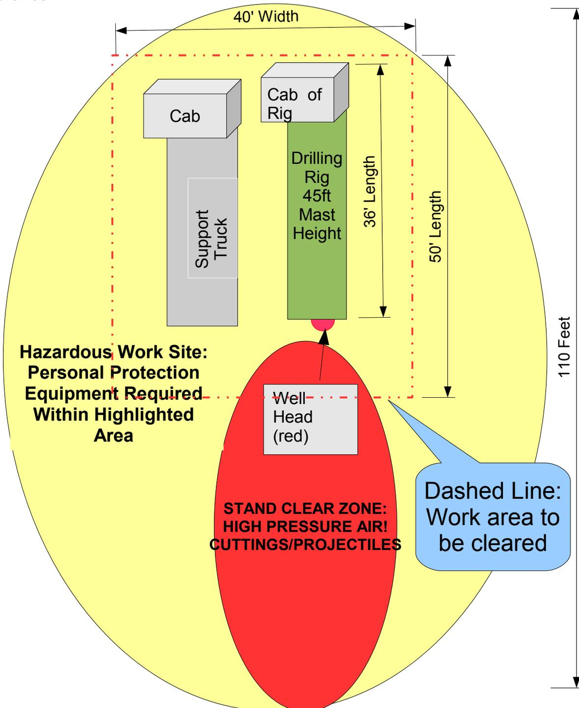
For additional cost, rig can be set up with optional cyclone discharge system - this will mitigate stand clear zone & projectiles.
